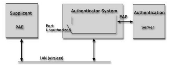
A Port Access Entity (PAE) is an entity that has access or is capable of gaining or controlling access to some port which offers some services. When applied to IEEE 802.11, the Access Point acts as an authenticator, while a wireless station (laptop etc) is the supplicant which is authenticated by the RADIUS server (Authentication Server).
